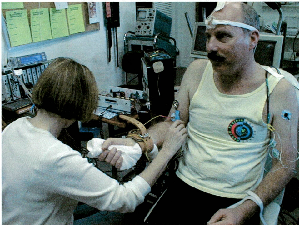
Figure 1. Testing for motor point location (MP) of the biceps brachii, after subject is positioned in the multipositional chair
